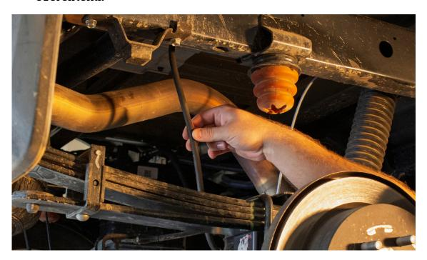
7: Install the lift block with the locating dowel facing down. Align the spring locating dowel with the hole marked "Frontier". Position the block with the Bear logo facing the rear.
