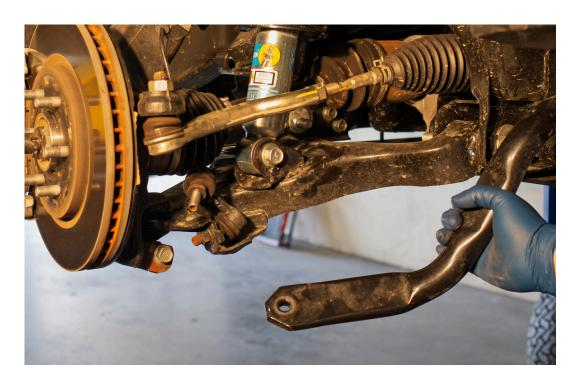
**Step 6:** Support lower control arm with floor or pole jack
