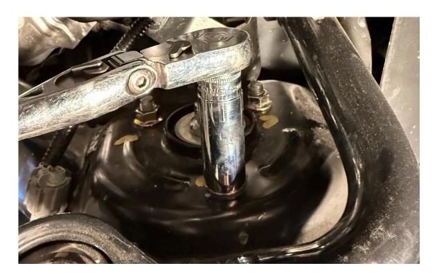
**Step 8:** Using 19mm socket and 19mm wrench remove the lower shock nut and bolt
