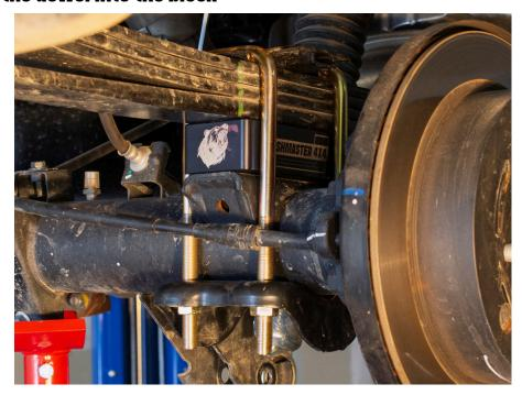
**Step 9:** Install the new U-bolts and the original U-bolt plate.
