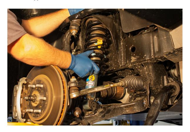
Then Pivot the shock away from frame, Lift up and out. (Be careful not to damage wheel speed sensor wiring or the fender during removal).
